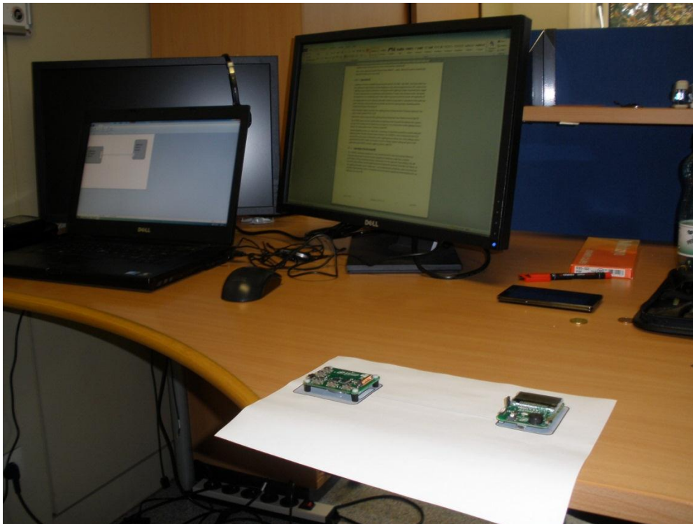
Figure 3: Distance of the DemoKit setup to other electronic devices for correct performance
