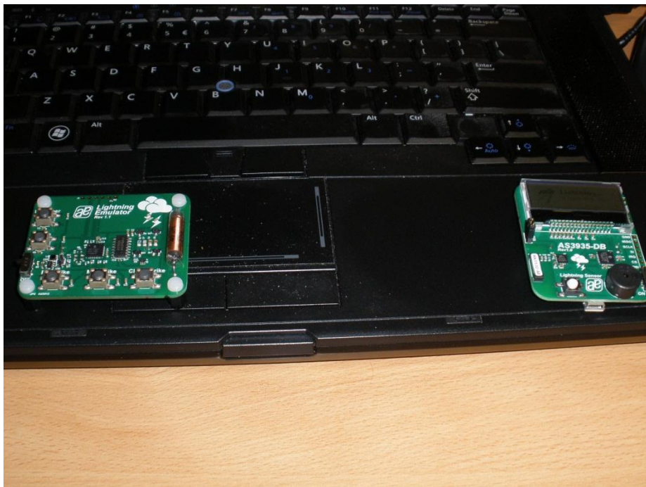
Figure 5: Although the Lightning Sensor Board might display 'Listening', its sensitivity is strongly influenced by the disturber and the DemoKit will not function correctly.
