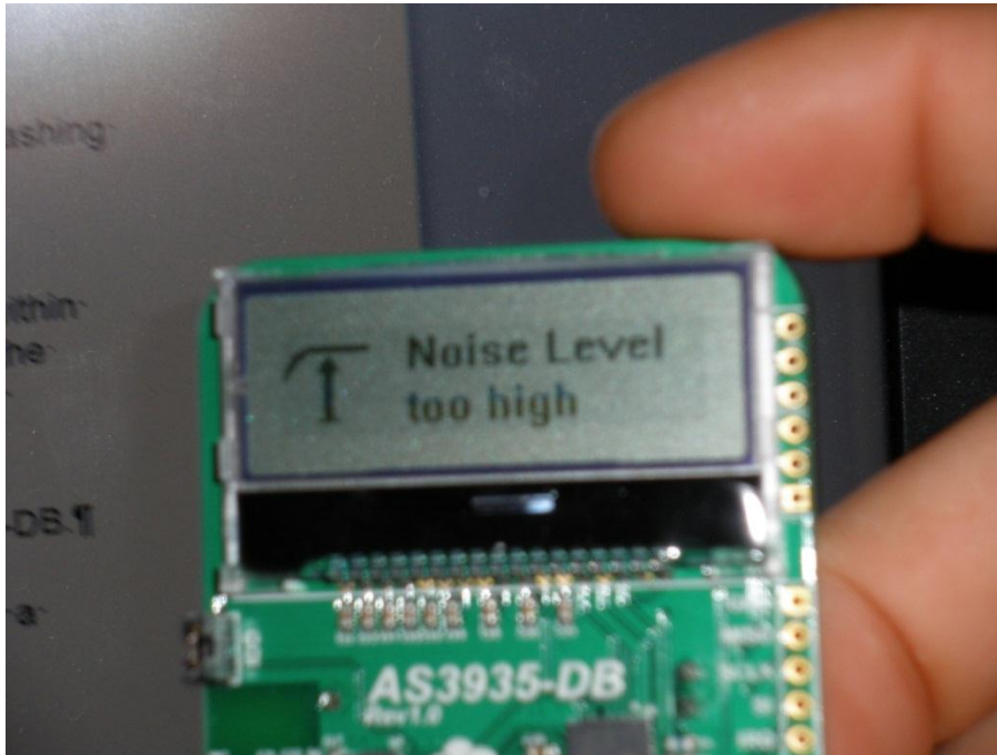
Figure 4: The noise level close to a LCD Screen is too high for correct operation.
