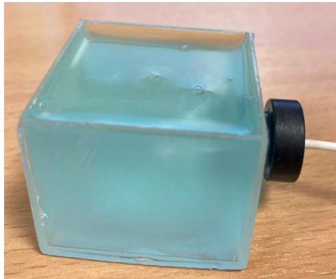
Picture 1: Container box with glued on transducer and filled up dish soap
