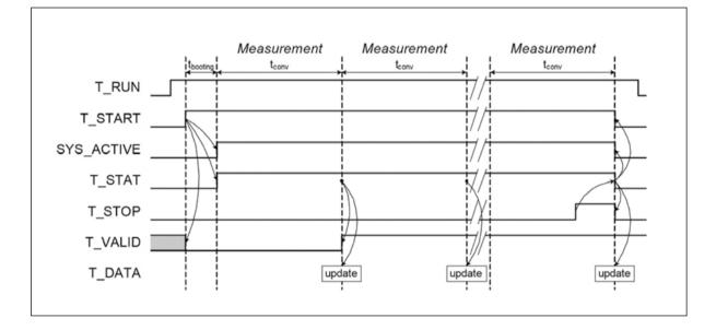
Signal T\_RUN is written high to select a continuous measurement. Note that T\_STOP is typically low (cleared by a previous measurement), and it should stay low otherwise continuous mode will stop after one measurement. T\_START is written high to start measuring: T\_VALID in T\_VAL is cleared and the device starts *booting* to *active*. Once *active* SYS\_ACTIVE goes high, and measurement starts (T\_STAT goes high).
