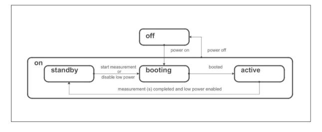
In continuous run mode (see Register SENS\_RUN) or when low power is disabled (see Register SYS\_CTRL), the device remains in *active* state.
