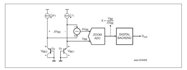
The temperature is measured using a high-precision (12 bits) zoom-ADC. The analog part is able to measure a strongly temperature dependent  $X = V_{BE}/\Delta V_{BE}$ . The X is found by first applying a coarse search (successive approximation), and then a sigma-delta in a limited range. The accuracy of the sensor is shown in Figure 12. The conversion time is shown in Figure 9.
