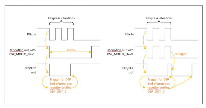
Figure 32: Port Trigger Timing
