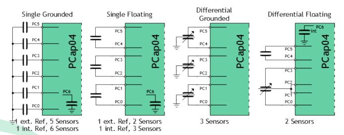
Figure 5: Connecting sensors
