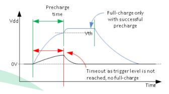
Figure 9: Short Circuit Detection
