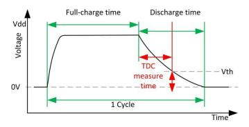
Figure 8: Single Cycle, Fast Charge
