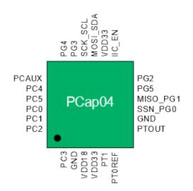
Package dimension: 4 x 4 mm<sup>2</sup> Suitable socket: e.g. Plastronics
