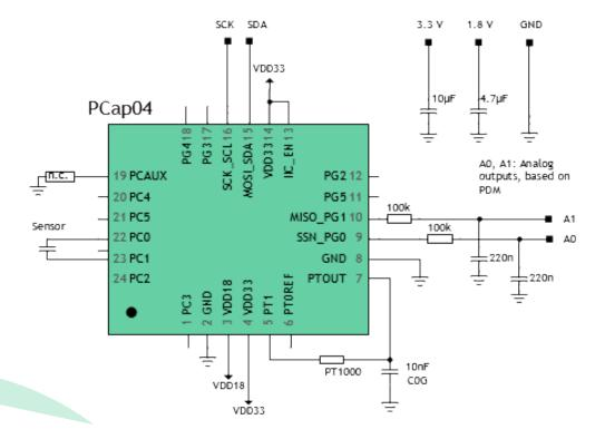
Figure 37: Typical Schematics with I<sup>2</sup>C Interface and PDM Analog Outputs
