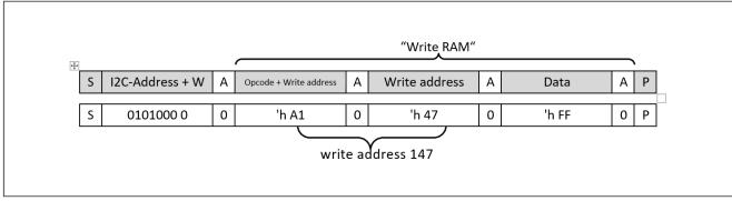
Example: Write 0xFF as a datum to the SRAM at address 0x147.
