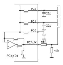
Figure 18: Guarding with Grounded Capacitors
