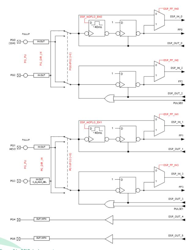
Figure 31: GPIO Assignment
