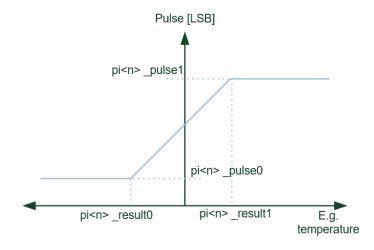
Figure 34: PWM and PDM Linearization
