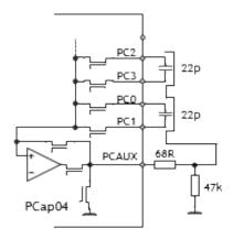
Figure 17: Guarding with Floating Capacitors
