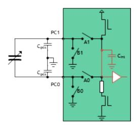
Figure 14: Internal Compensation Measurement
