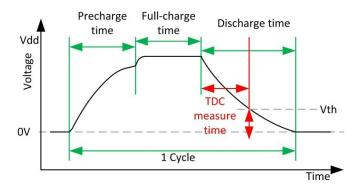
Figure 7: Single Cycle Timing
