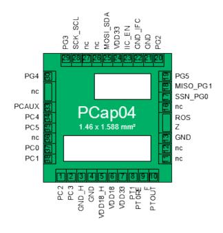
Figure 2: Pin Diagram of PCAP04 Die
