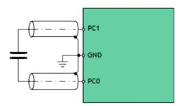
Figure 15: Shielded Cables
