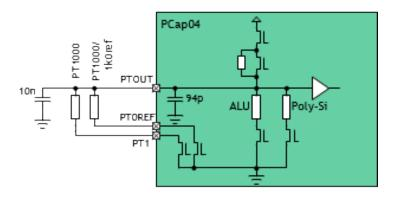
Figure 21: Connecting Temperature Sensors
