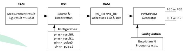
Figure 33: PWM and PDM pulse generation
