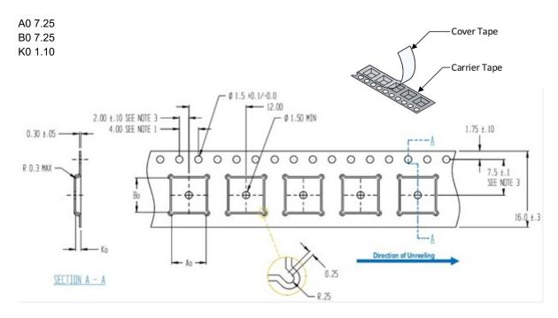
Figure 44: Carrier Tape QFN24
