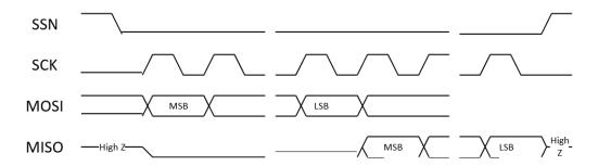
Figure 30: SPI Read Procedure
