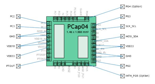
Figure 38: 2-Side Bonding
