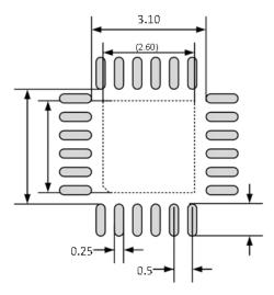
Figure 41: Landing Pattern (dimensions in mm)
