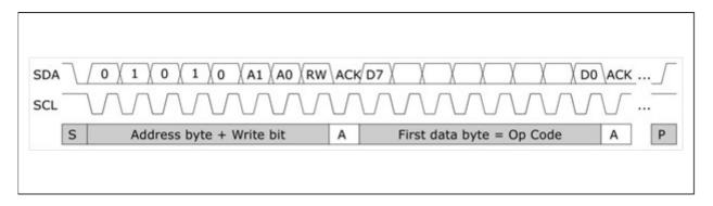
Figure 26: I<sup>2</sup>C Typical Sequence
