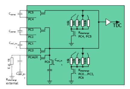
Figure 6: Integrated Discharge Resistors
