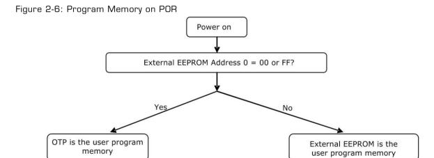
Once the user program development is completed using the external EEPROM then, the final program is ready to be written to the OTP. Then the external EEPROM is either removed physically or it is made inactive to the PSØ9 by writing the address OO of the external EEPROM with OO or FF. The following flowchart gives an overview of how the user program is developed using the EEPROM and transferred to the OTP finally.
