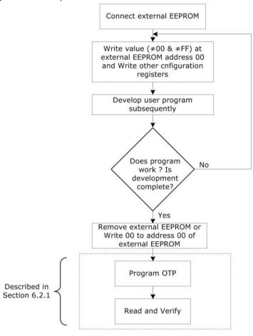
The PSØ9 Assembler Software which is used for user program development supports downloading the developed program to the external EEPROM or to the on chip OTP. The target for downloading the program can be selected from a drop down list on the Download page of the assembler.
