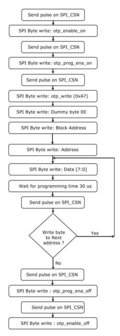
For a list of all op codes pertaining to accessing the OTP through the SPI / IIC interface, refer to Vol.1, Chapter 4, section 4.5.3.3 OTP Access.
