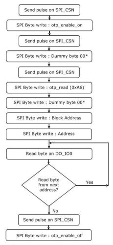
st the Dummy byte (0x00) is required to be sent as it is needed because of timing purposes
