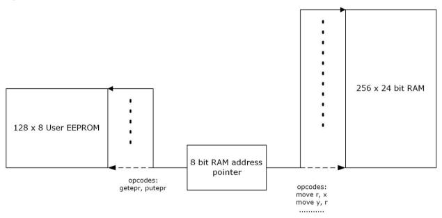
When the RAM address pointer is set to a value and op codes putepr and getepr are used, the RAM address pointer points to the respective byte in the user EEPROM. Hence operations are carried out with the respective user EEPROM byte. All other op codes like move r, x set the RAM address pointer to point to the RAM, hence the operation is performed in the RAM.
