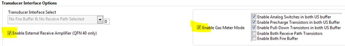
With this setting, general purpose IOs GPIO0, GPIO1, GPIO4 and GPIO6 provide the signals to control external analog switches.
