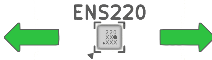
Figure 12. The device is more resistant to deformations from the direction of the green arrows (horizontal in the picture) than in other directions.
