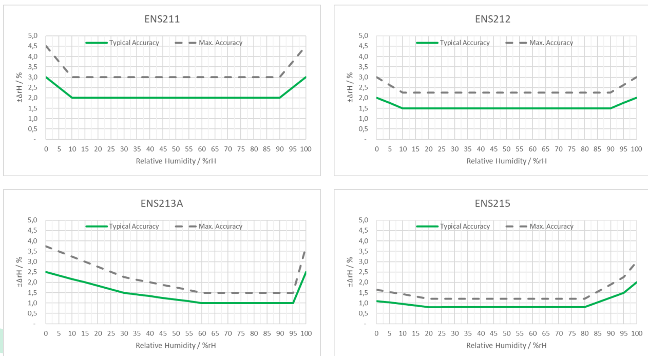
Figure 7: Relative humidity sensor accuracies 11
