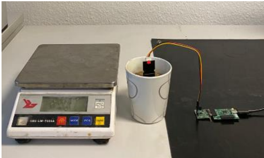
Figure 9 Test Setup (Probe Inserted into Soil, Weight Scale and PCAP04 Evaluation Kit)
