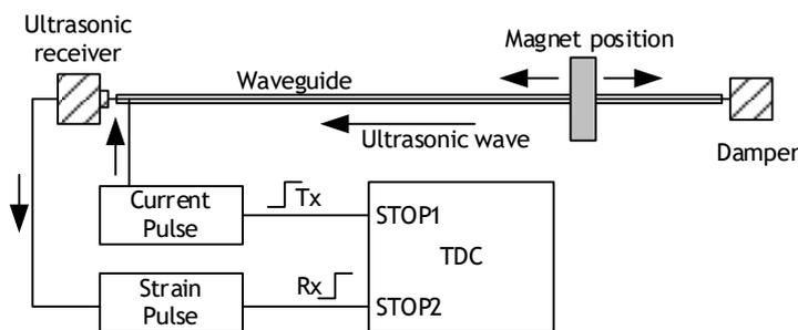
Figure 1: Basic components of magnetostrictive sensor
