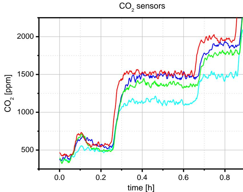
Figure 5: Device-to-device variation of NDIR CO<sub>2</sub> sensors of the same type and age
