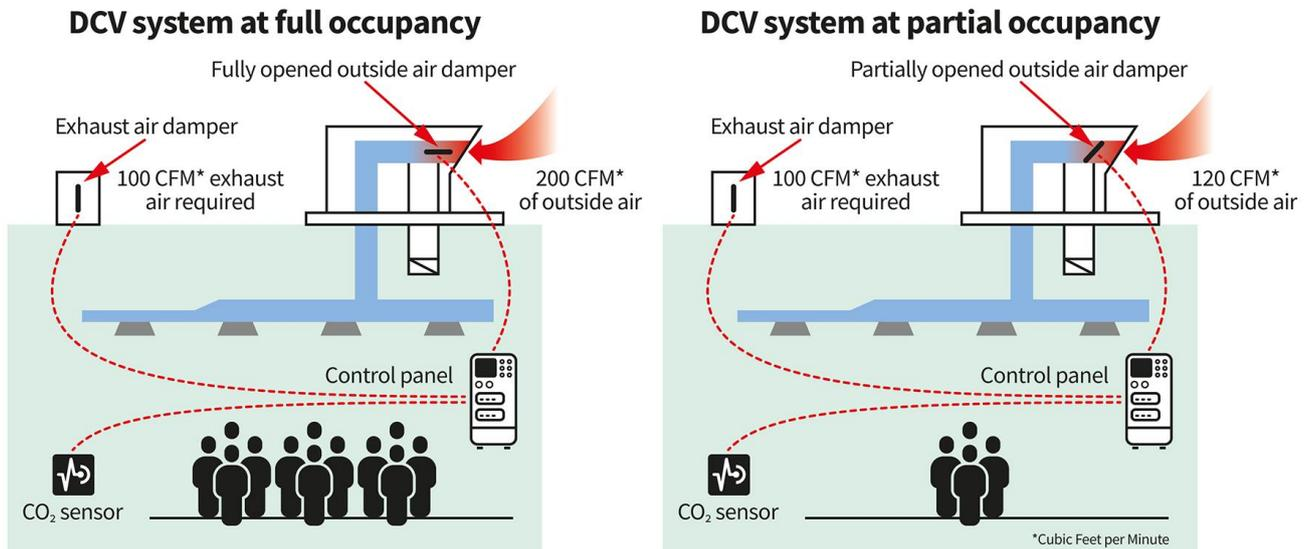
Figure 2: CO<sub>2</sub>-regulated DCV systems.
