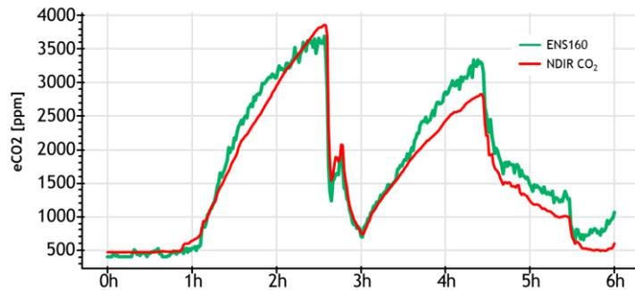
Figure 3: Comparison between SciSense ENS160 eCO<sub>2</sub> readings and NDIR CO<sub>2</sub> outputs.
