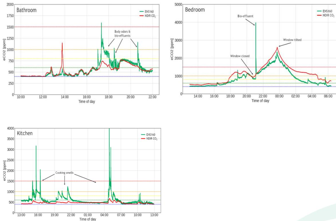
Figure 4: eCO<sub>2</sub> reading of a SciSense VOC sensor compared to NDIR CO<sub>2</sub> selective sensor. The VOC sensor detects body odors and bio-effluents common in bathroom, bedroom and kitchen environments which are not detected by a selective NDIR CO<sub>2</sub> sensor.
