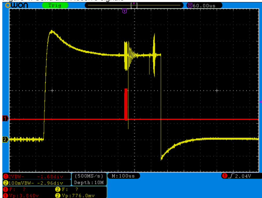
Figure 4: Send and Receive signals
